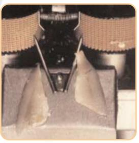
The Pisces FR-150 and FR-200 are reliable, versatile, high-speed filleting units specially designed for the production of single fillets free of backbone and ribs. Only minor adjustments are required to process a wide variety of fish species and sizes due to the machines' unique location method that utilizes the internal bone structure of the fish.
